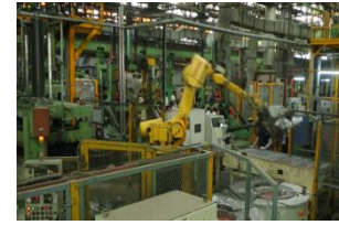
Gravity die casting cell
